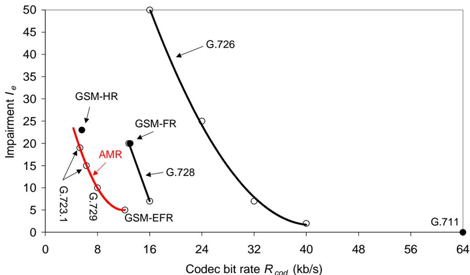
**Figure 4: Impairment  $I_e$  for several standardized codecs. The points are experimental rate-distortion pairs. Based on this experimental input the rate-distortion (codec bit rate  $R_{cod}$  vs. Impairment  $I_e$ ) curve is interpolated for the G.726 codec, the G.728 codec and the AMR codec.**
