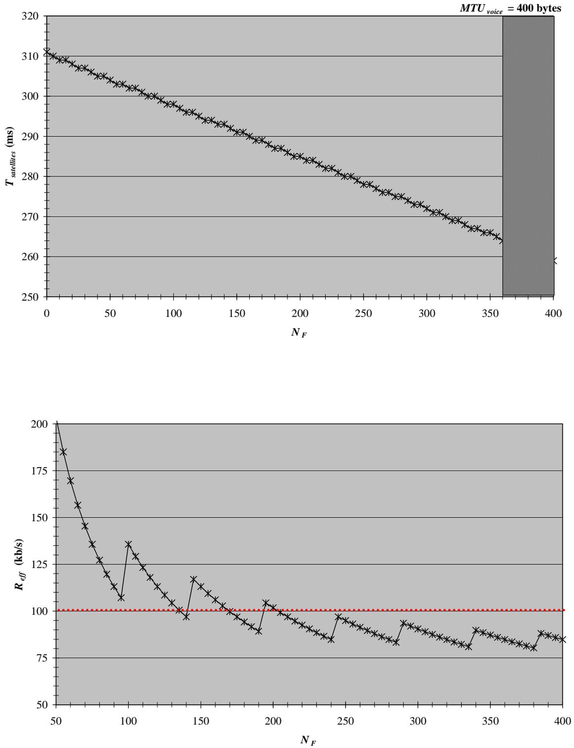
**Figure 5: The satellite delay budget  $T_{satellites}$  and the effective bit rate  $R_{eff}$  as a function of the number of voice code words for the **G.711@64 kb/s** codec, a packet loss ratio of 0.1 % and an echo loss value of infinity.**
