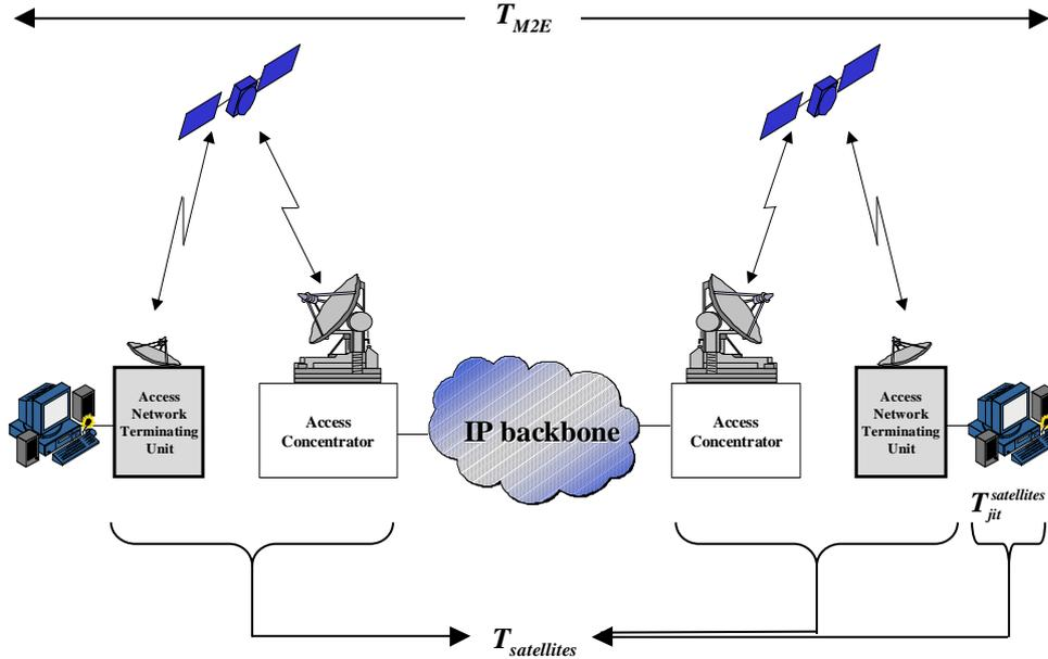
**Figure 4: The satellite-PC-to-satellite-PC VoIP scenario.**
