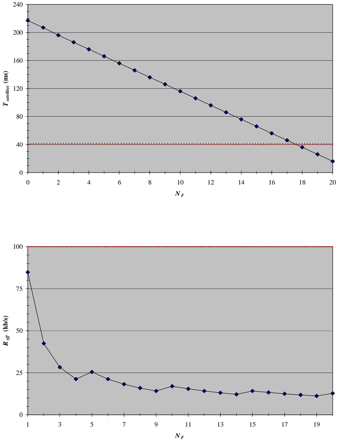
**Figure 8: The satellite delay budget  $T_{satellites}$  and the effective bit rate  $R_{eff}$  as a function of the number of voice code words for the **G.729@8 kb/s (+VAD)** codec, a packet loss ratio of 0.1 % and an echo loss value of infinity.**
