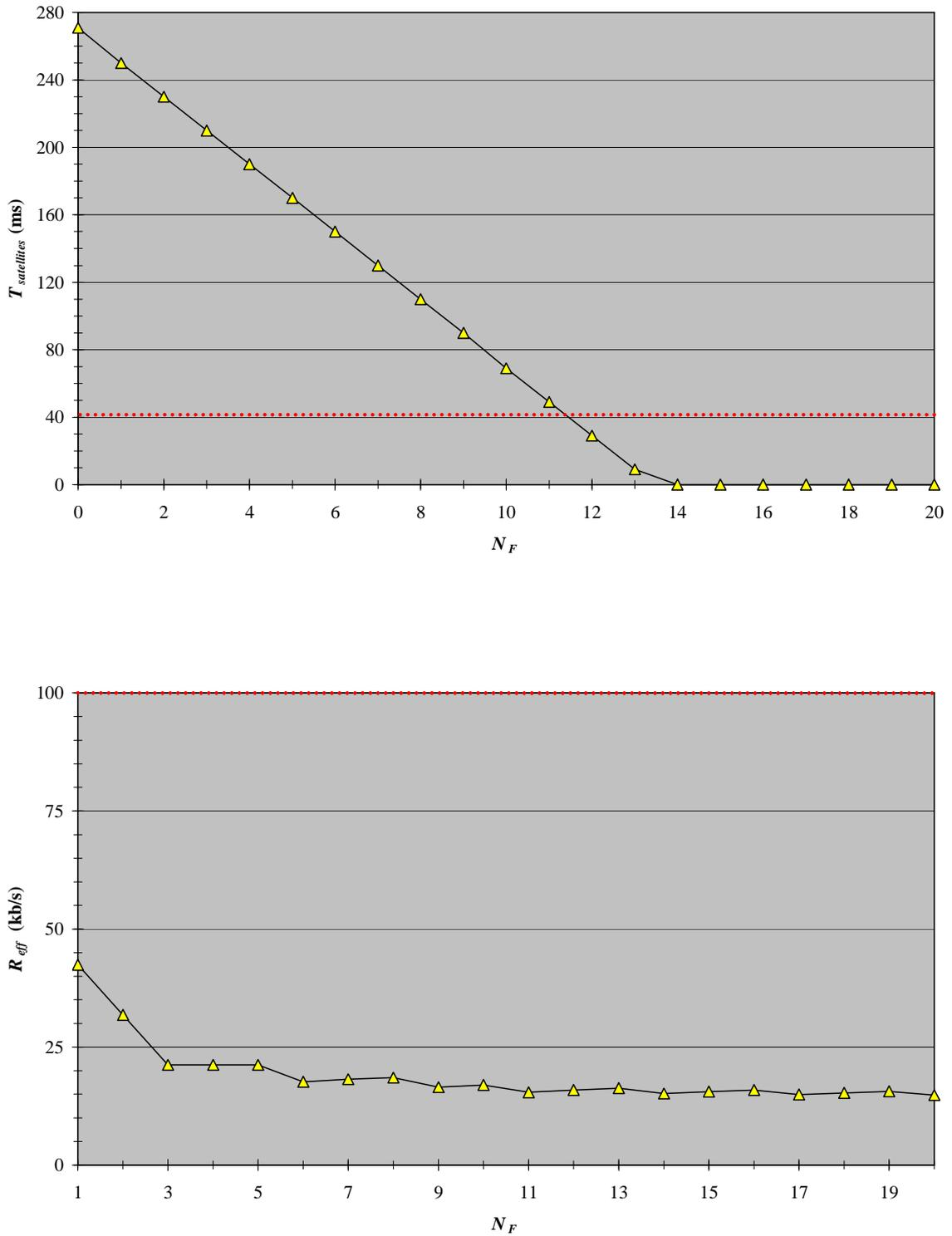
**Figure 7: The satellite delay budget  $T_{satellites}$  and the effective bit rate  $R_{eff}$  as a function of the number of voice code words for the GSM-EFR@12.2 kb/s codec, a packet loss ratio of 0.1 % and an echo loss value of infinity.**
