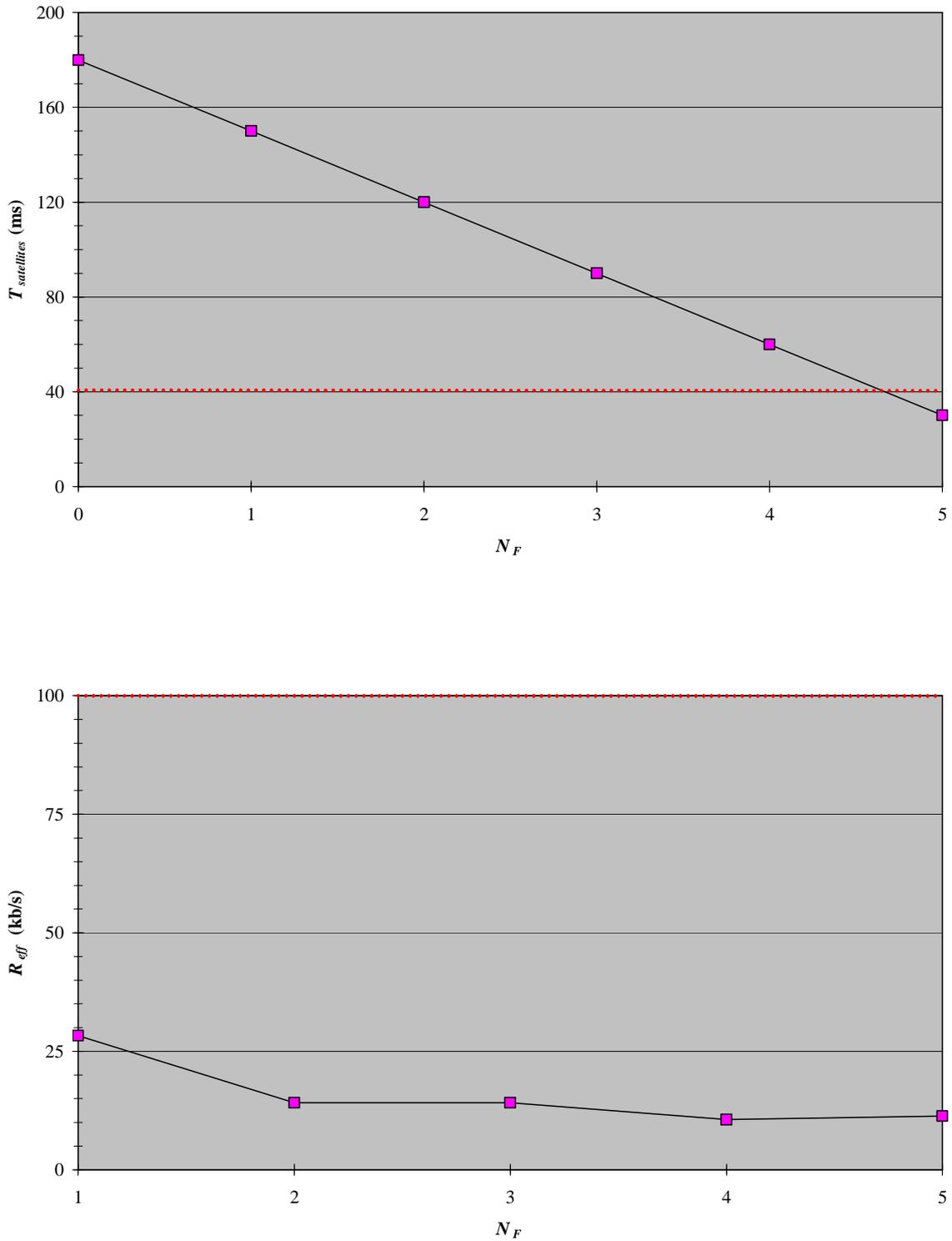
**Figure 9: The satellite delay budget  $T_{satellites}$  and the effective bit rate  $R_{eff}$  as a function of the number of voice code words for the **G.723.1@6.3 kb/s (+VAD)** codec, a packet loss ratio of 0.1 % and an echo loss value of infinity.**
