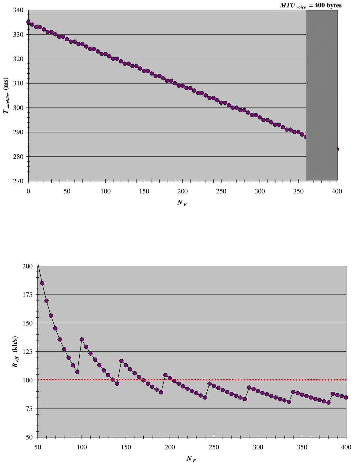
**Figure 6: The satellite delay budget  $T_{satellites}$  and the effective bit rate  $R_{eff}$  as a function of the number of voice code words for the [G.711@ 64 kb/s (+PLC)] codec, a packet loss ratio of 0.1 % and an echo loss value of infinity.**
